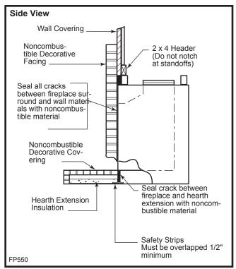
Fig. 25 Sealing gaps.
